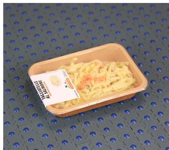
Another important aspect is the total weight of the good: most of the times is suitable with the max working load of the belt, especially of the spheres. Anyway, we always suggest to double check that the total weight of the good does not exceed the max load of the spheres, **15N/ea.**
