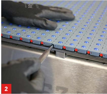
Insert a pin punch and push to extract the white rod from the opposite side.
